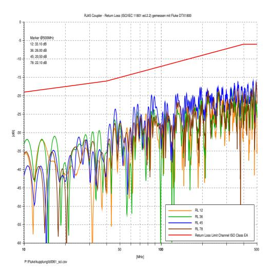
The return loss test result of all pairs shows significant headroom with respect to the specified values. There are neither visible artifacts nor deterioration patterns which could be attributed to the presence of the couplers.
