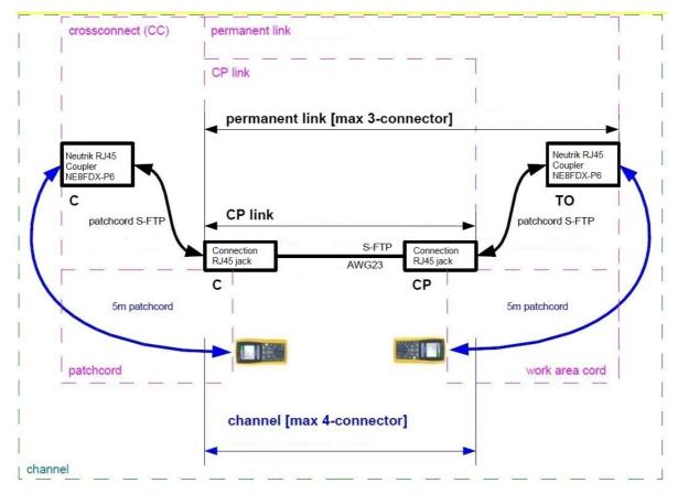
Test setup with Fluke DTX-1800 with all components and couplers shown. The length of the S-FTP AWG23 solid cable is 15 m. All patch cords are AWG27/7 stranded cable with a length of 5 m.
